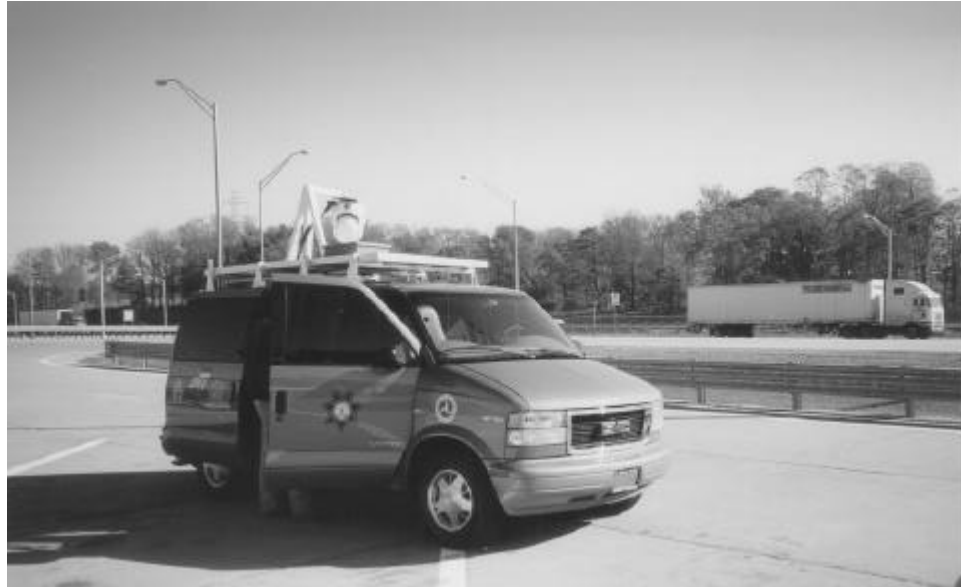
Figure A-3. The IRISystem, set-up at a scale site in Kentucky.
