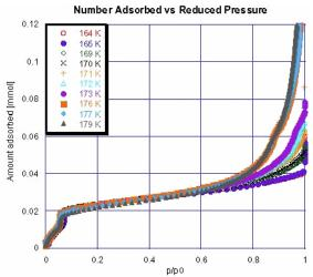
Figure 1: Methyl Bromide on MgO isotherms measured at set-point temperatures of 164 K to 179 K. Actual temperatures are determined using the saturated vapor pressure for MeBr at the set-point temperature.
