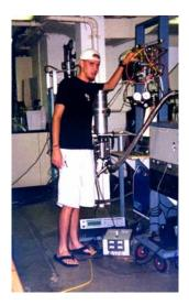
Undergraduate TJ Harper makes adsorption measurements; shown is the gas handling system, the helium cryostat, and vacuum system. Work was completed in Dr. John Larese's lab at the University of Tennesee.
