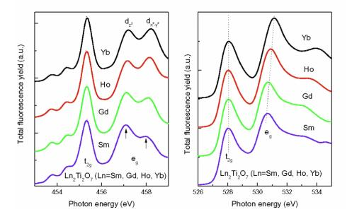
Ti 2p (left) and O 1s (right) NEXAFS spectra from  $\text{Ln}_{2} \text{Ti}_{2} \text{O}_{7}(100)$  (Ln=Sm, Gd, Ho and Yb) single crystals.
