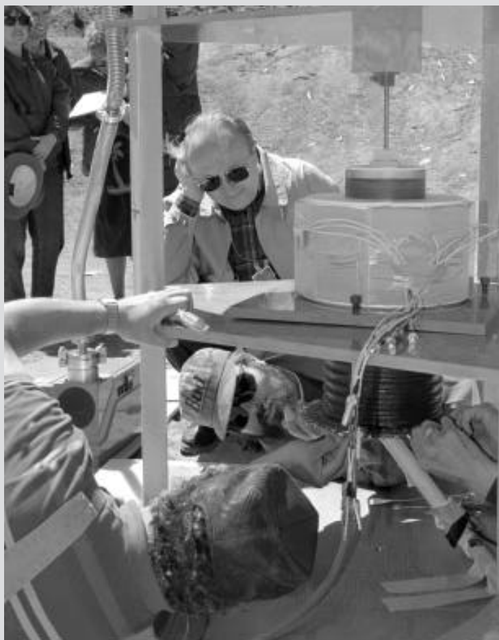
Preparing for the experiment. Mikhail Dolotenko of Arzamas-16 (kneeling), oversees the installation of his samples and diagnostics into the bore of the MC-1 flux compression generator (oriented vertically for this experiment). Lying down are Los Alamos technicians Tommy Herrera (facing) and Dave Torres.
