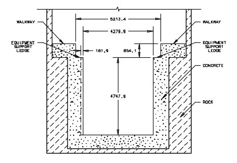
Figure 4.2-35 Target hall pit cross section
