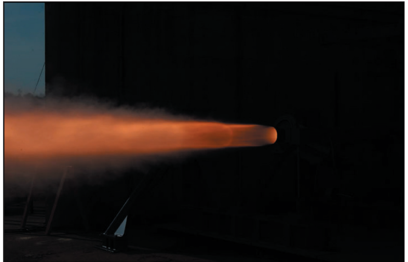
An exhaust plume is produced during a space shuttle booster separation motor test at the Marshall Center Feb. 17. The 1.2-second motor test achieved the expected maximum thrust, 23,000 pounds force, and met the test objective of proper test stand installation.
