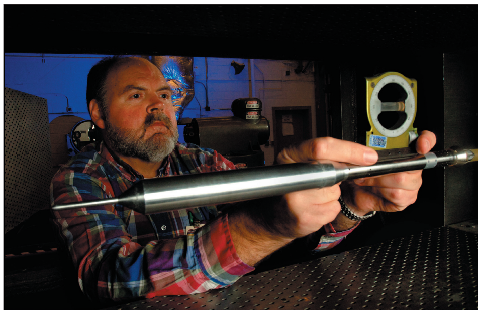
Test engineer Alonzo Frost with a Crew Launch Vehicle model being tested in the Marshall Aerodynamics Research Facility.
