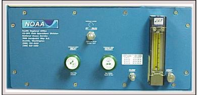
**Figure 5: Front of Pressure Control Panel**
