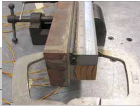
TF Coil Weld Test 4-30-08 w/ Heat Sink
