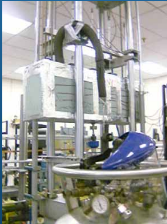
Sealed Insulation box with test bar Inside
