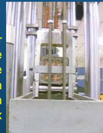
Bar Fitted with Probes for Electrical Testing after Cycling
