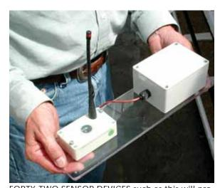
FORTY-TWO SENSOR DEVICES such as this will provide a stream of data to researchers on temperature, humidity, light intensity, and barometric pressure at multiple sites throughout the greenhouse.
