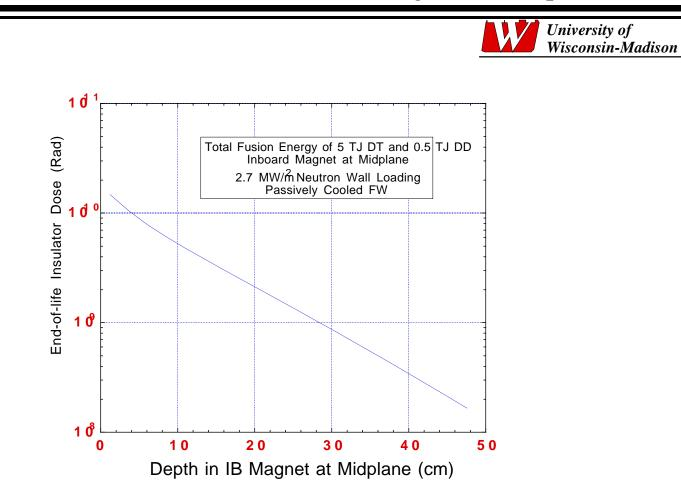
• Peak end-of-life insulator dose drops to  $10^{10}$  Rads behind the front 4 cm layer of the coil
