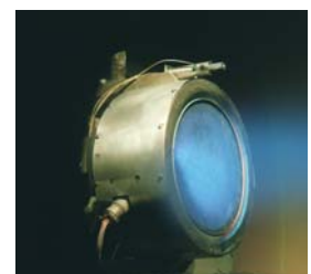
Ion engine used on the Deep Space 1 spacecraft
