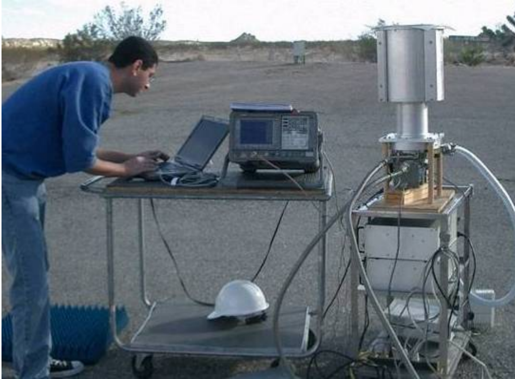
Figure 8 – Test setup for noise measurements of the cooled feed at Goldstone on Oct 10, 2006 using cold sky and absorber (lower left) on top of the feed window.
