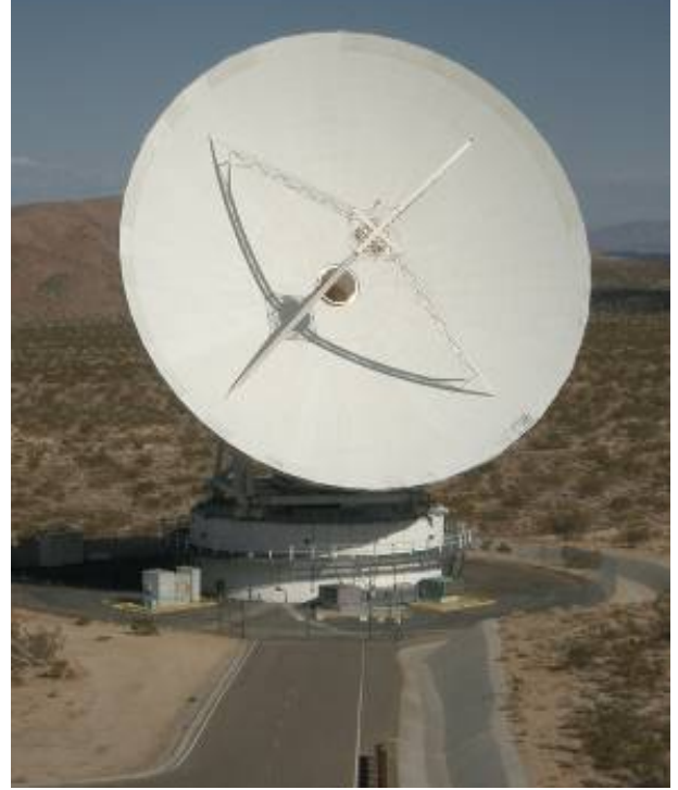
Figure 1 – Photographs of the DSS27 antenna which is identical to the DSS28 which will be modified for the wide band operation described in this paper. The original antenna has a beam-waveguide optical system which guides the beam through the 2.74m diameter hole at the vertex, through mirrors, to a large stationary control room in the antenna base. The revised system will utilize a tertiary reflector covering hole with receivers located near the vertex.
