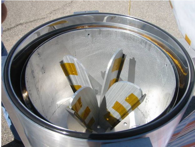
Figure 5 – Feed in dewar and in pattern test chamber. The feed patterns were tested with a surrounding cylinder at upper left, the cylinder lined with absorber at upper right, and in the cylinder but with absorbing strips taped to the outer rim as in lower left. All pattern measurements were made in a small chamber at Caltech as shown in lower right, where in this photo, the feed without cylinder or absorber was tested. The efficiency calculations were performed from pattern measurements with the feed with absorber strips and in a cylinder as in lower left
