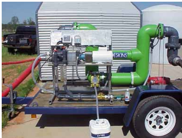
Figure 2. The in-line PAM injector and mixer used in the pilot study to flocculate the solids in the flushed manure. A polymer feed system (foreground) was used to dilute and prepare the polymer before injection into the in-line static mixer (background), where diluted polymer was mixed with the flushed manure.
