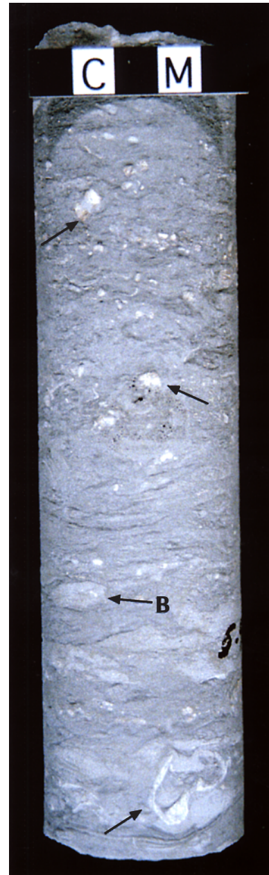
Figure 2.24. Core section showing nature of fossiliferous siltstone facies. Fossil fragments are white (arrows) in core and the siltstone is blocky to massive. Also visible are horizontal burrows (B); (locality C5).
