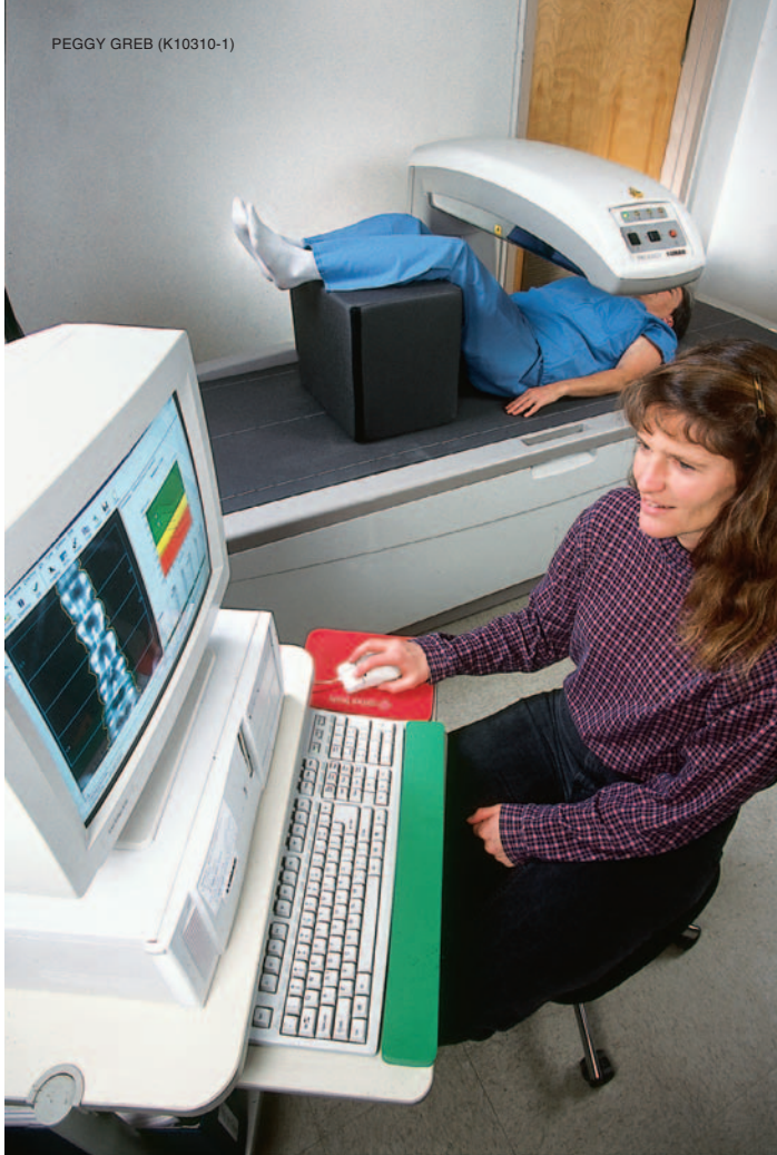
Using DXA (dual energy x-ray absorptiometry), physiologist Mary Gustafson-Storms makes a bone density measurement of the spine of a research volunteer.
