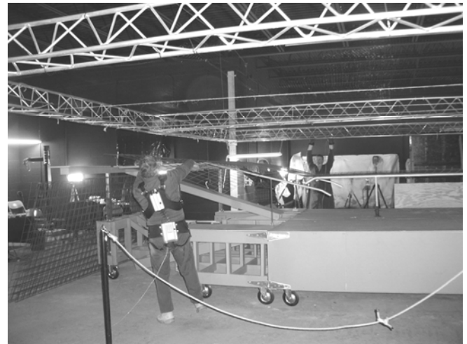
Figure 9. Full scale wooden mockup of bolter with rails that permit sliding of screen across canopies.
