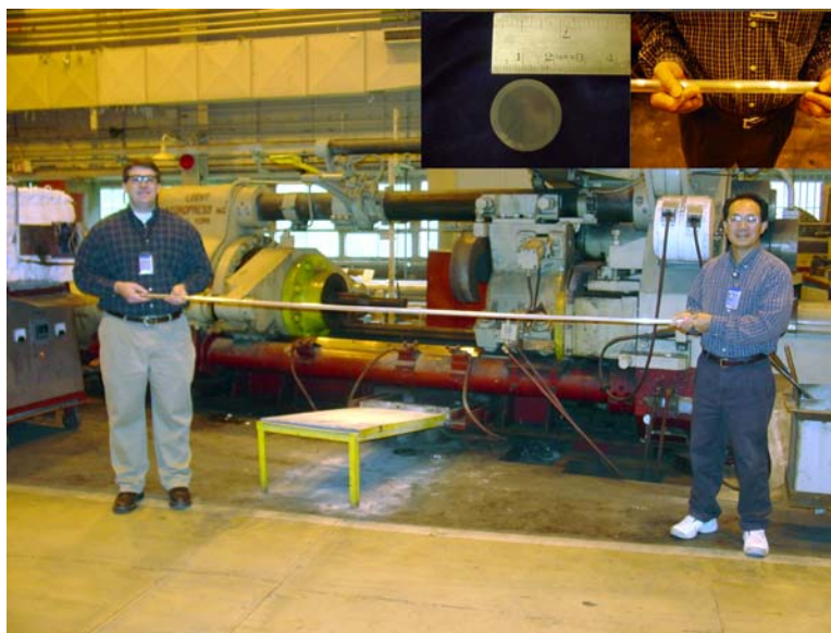
Figure 2.2.3: Photograph of the 7075 baseline alloy extrusion and (top right) a cross section indicating no gross porosity.
