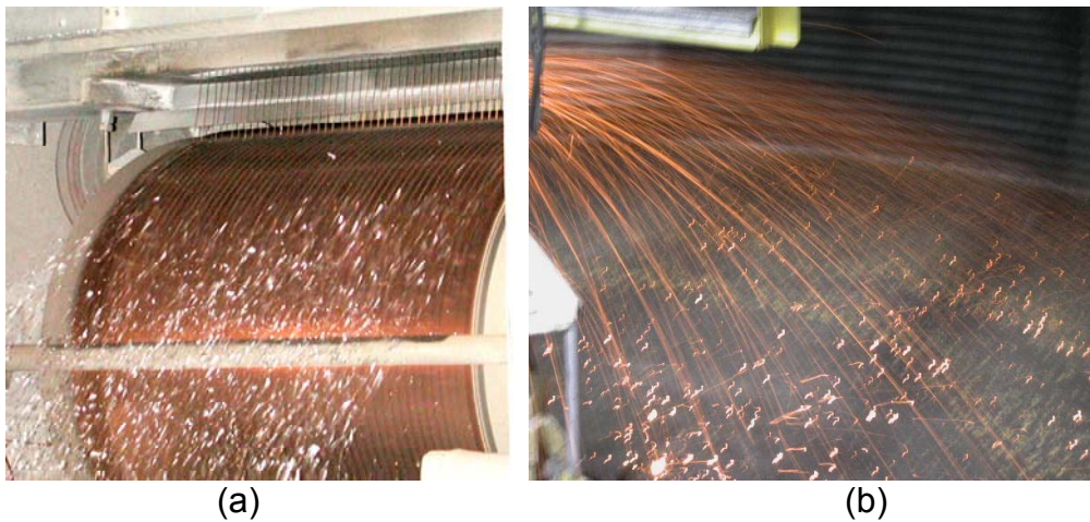
Figure 2.1.7: Transmet rapid solidification processing showing (a) melt spinning of flake, and (b) centrifugal atomization (Courtesy of Transmet Corporation).
