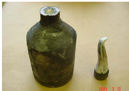
Figure 2.2.4: Photographs of the unsuccessful Al-Mn extrusion at the can side (left) and at the extruded side (right) after removal from the extrusion die.
