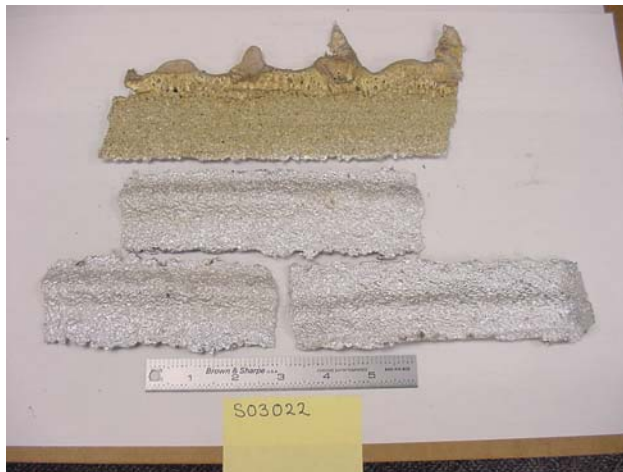
Figure 2.2.2: Typical view of a splat quenched 2219 + Al 2 O 3 alloy.
