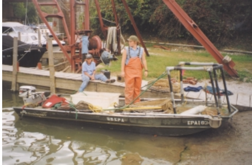
Figure 2-4. A jon boat heavily loaded with sampling equipment. This illustrates the need for boats with deep sides.
