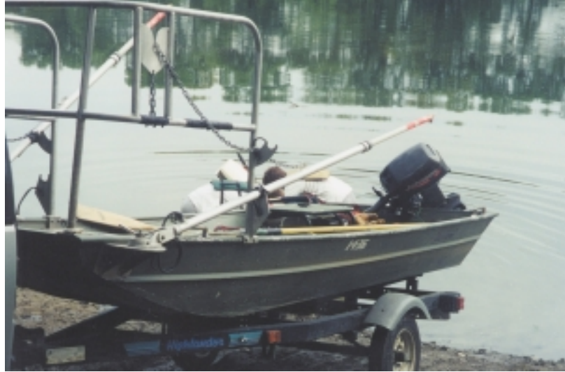
Figure 2-1. An example of a jon boat, trailer and outboard motor.
