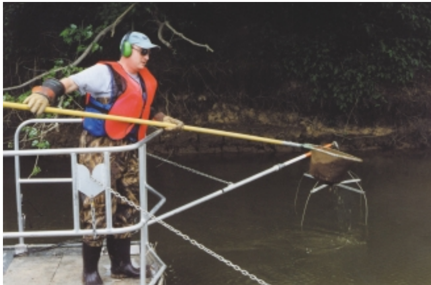
Figure 3-1. A member of a field crew removes fish from the river during a fish sampling effort in which electroshocking equipment is being used. Note that the crew member is wearing hearing protection, eye protection, a life jacket, an orange safety vest, protective gloves and protective waders. The gloves and waders help to protect the crew member from electric shock.
