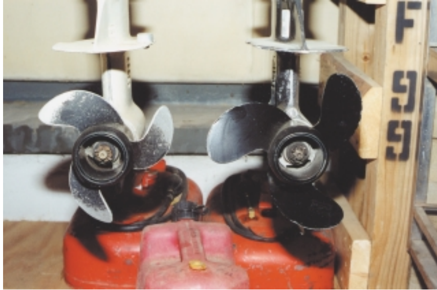
Figure 2-12. An excessively worn propellor (left) is contrasted with a relatively unworn propellor (right).
