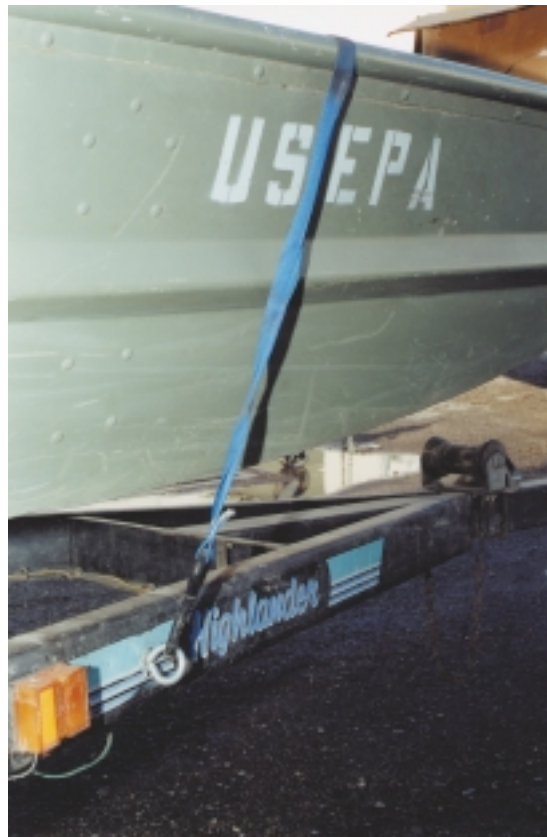
Figure 2-9. An eye bolt has been added to this trailer. This simple modification allows the boat to be securely fastened to the trailer with a ratchet strap so that the boat can be safely transported..
