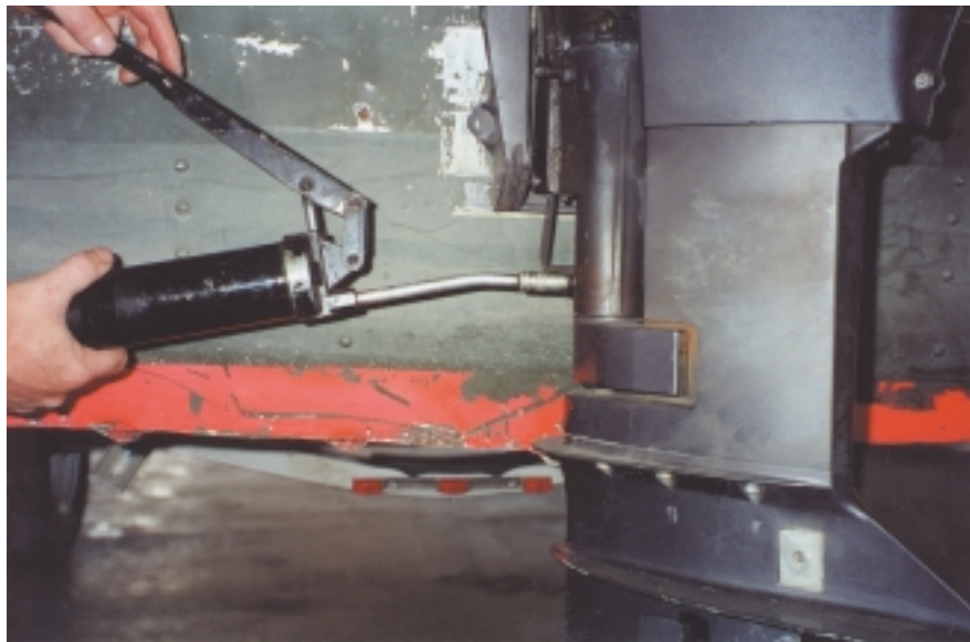
Figure 2-10. An outboard motor being lubricated.
