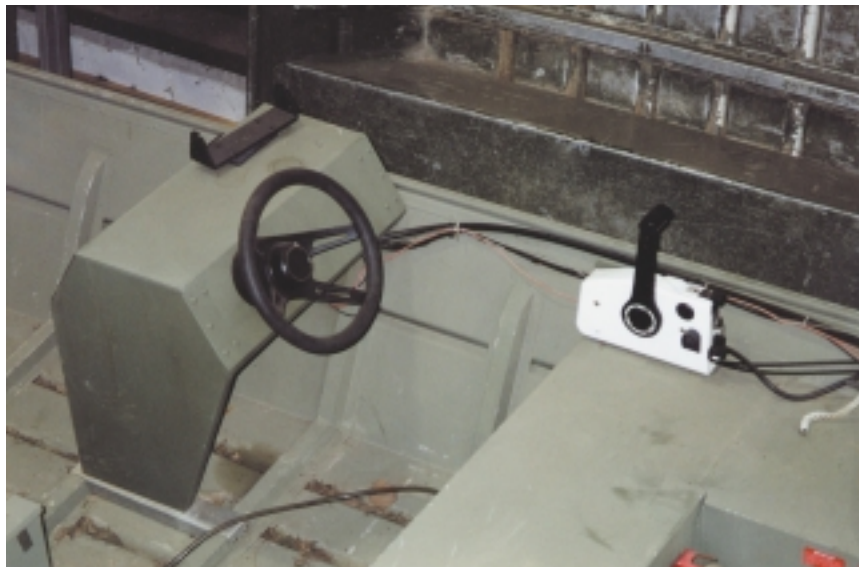
Figure 2-5. A jon boat with a steering console.
