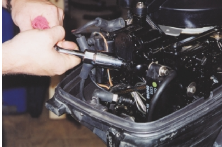
Figure 2-11. A spark plug being removed from an outboard motor.
