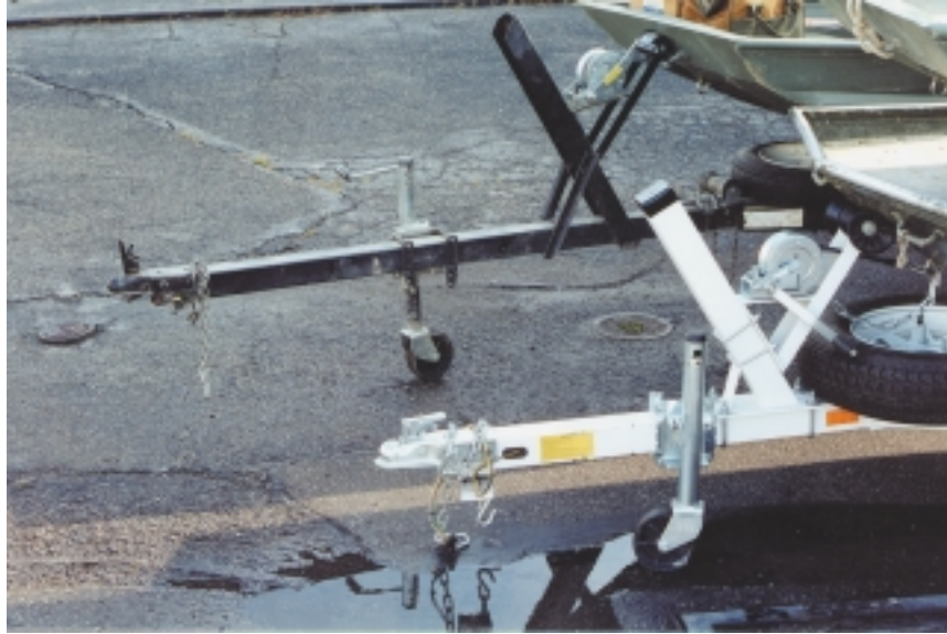
Figure 2-8. A long neck trailer (background) is contrasted with a short neck trailer (foreground). Note that the spare tires for the trailers are mounted horizontally on the trailers.
