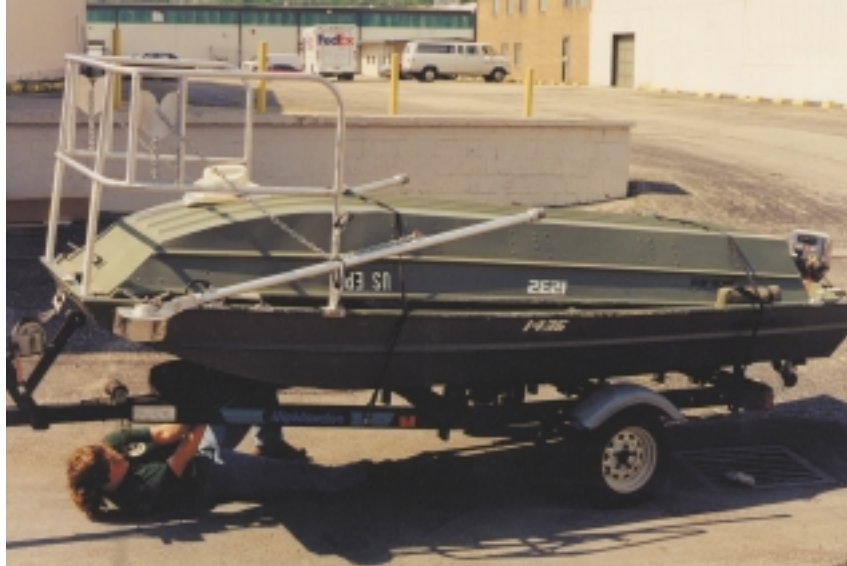
Figure 2-3. A smaller jon boat inverted and placed on top of a larger jon boat. This is an efficient method for transporting two boats to the same sampling site.
