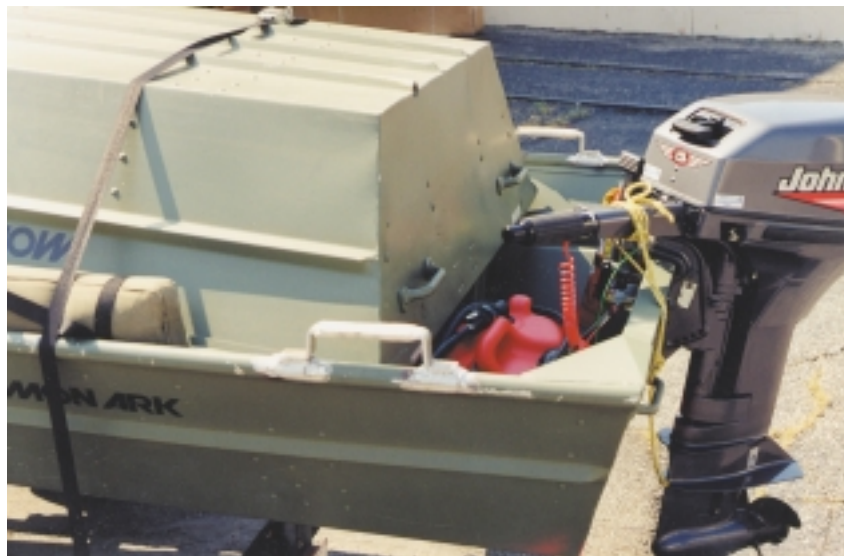
Figure 2-6. A jon boat that has had handles added to it. These handles allow field crews to more easily maneuver the boat when it is in shallow portions of a stream or river or when the boat is not on the water.
