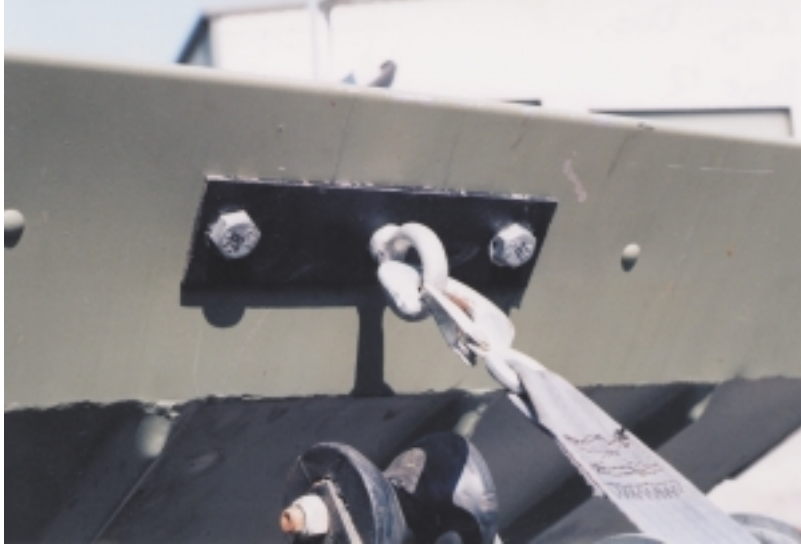
Figure 2-7. A jon boat with a reinforced bow eye. The fortification of a bow eye can help protect the boat from damage and help prevent injuries and accidents.
