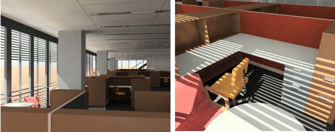
Figure 1 Work in progress to develop automated interior shading control, glare control, and daylight dimming lighting controls for an all glass façade in New York City. The Radiance simulation program ( radsite.lbl.gov ) is used to simulate the dynamic performance of interior operable shading with fixed exterior sun control elements, for different orientations; results will be used to develop shade control strategies.
