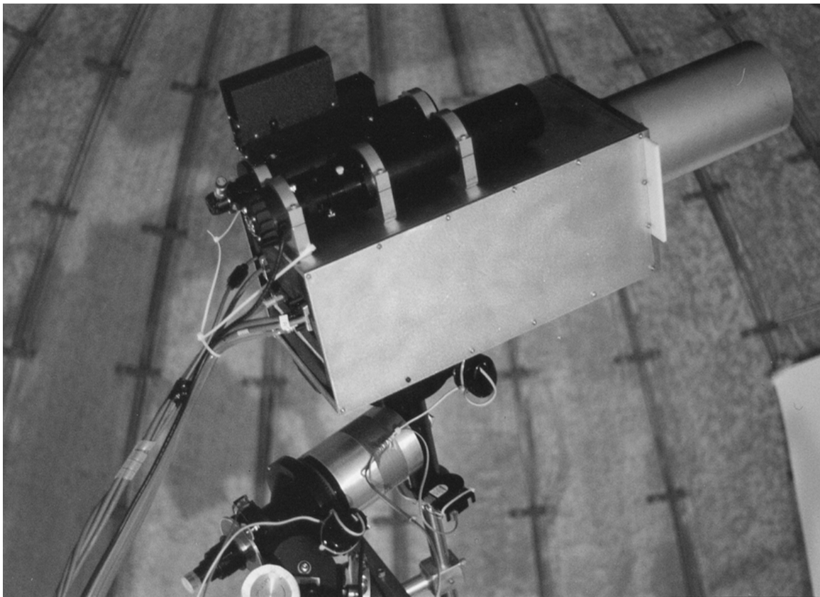
Figure 3. Photo of the Vulcan Photometer in the Crocker Dome. At the top are two finder scopes and auto guider. The white rectangle at the base of the tubular light baffle is the diffuser plate used for flat field calibration.
