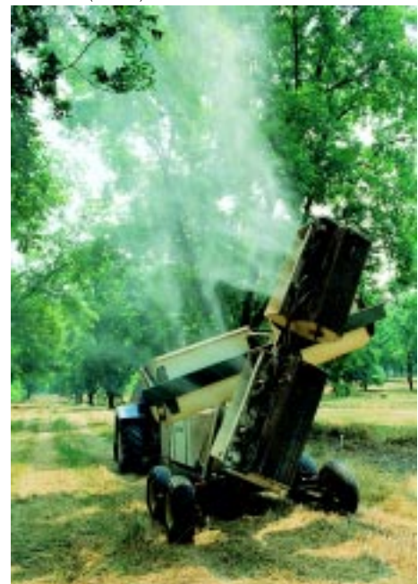
This new nozzleless sprayer uses one-half to two-thirds less spray to achieve superior coverage and penetration of the tree canopy.
