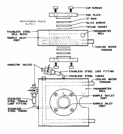
FIGURE 2. Stainless steel absorption cell.
