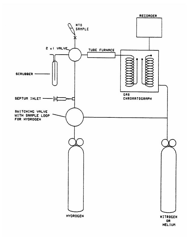
FIGURE 4. Water equivalent apparatus, schematic.
