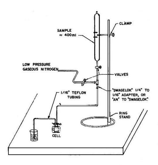
FIGURE 1. Nitric oxide sampler apparatus.
