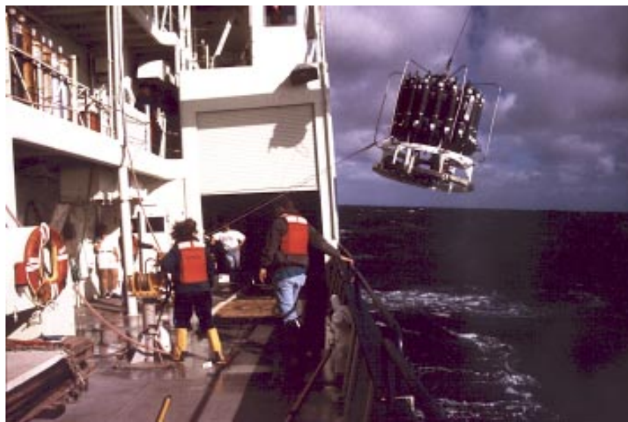
During the recent research cruise that BNL participated in on the Indian Ocean, crew members of the R.V. Knorr bringing the deep ocean water sampler aboard off the coast of Madagascar. In the sampler, 36 separate 10-liter bottles close at different depths as a result of cable signals from on board the Knorr.
