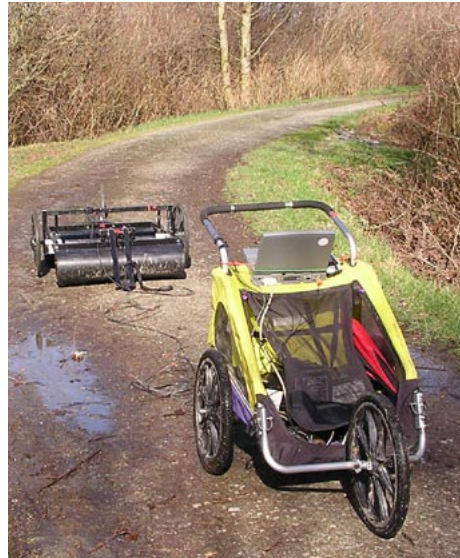
Ground-penetrating-radar system. Transceivers and receivers are towed on a cart behind a handpushed buggy carrying the data-acquisition equipment, including power supply, electronics, and laptop computer. This system is effective for imaging the subsurface over large distances in areas with little or no vegetation. The instruments can also be carried by hand over more rugged or highly vegetated terrain.
