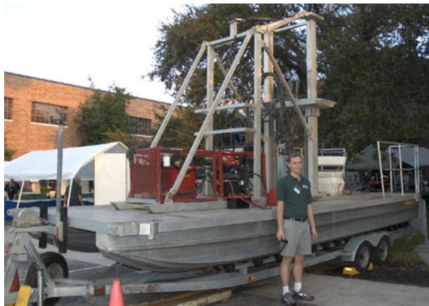
Geologists Chris Reich (not pictured) and Jason Greenwood (beside barge) assembled the auger-drill barge to show how cores are drilled in sand and clay. The auger drill has a corkscrew-shaped drill.
