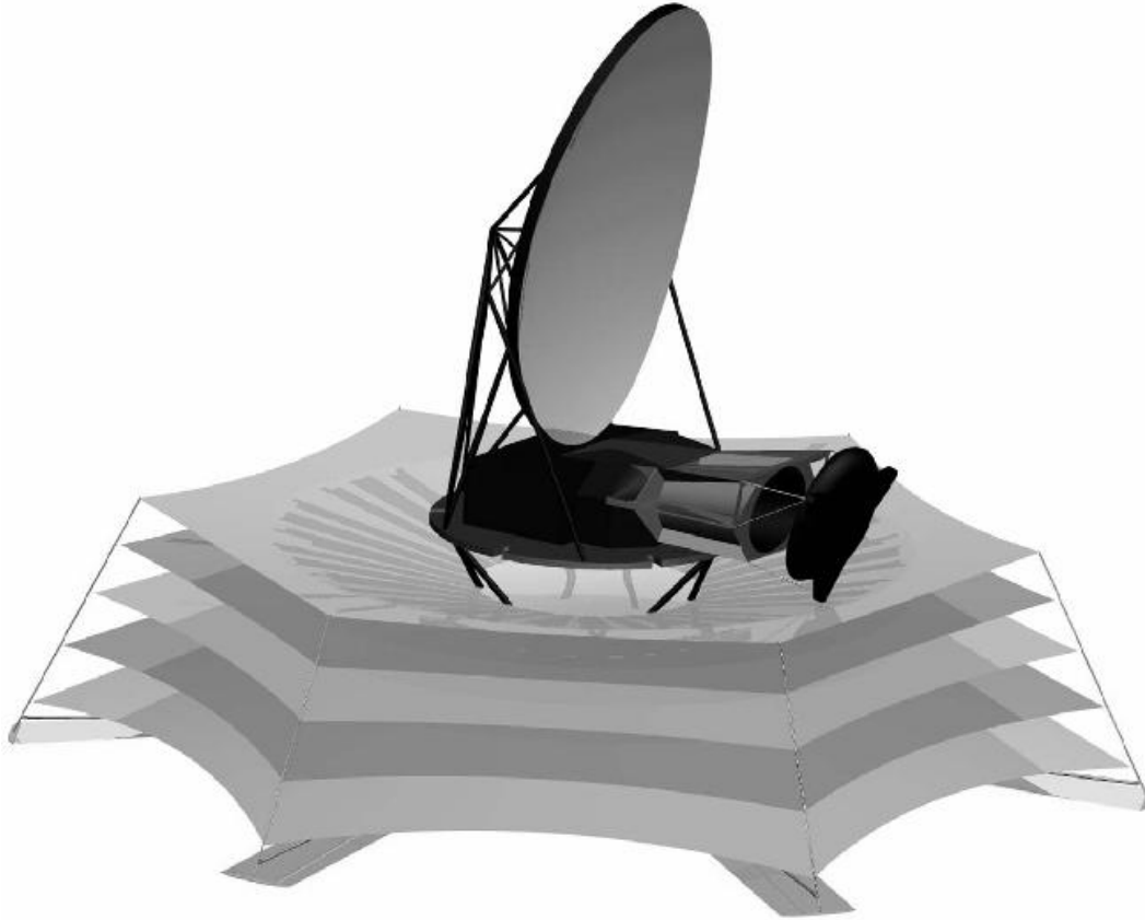
Figure 11. View of CALISTO spacecraft showing primary and secondary reflectors, cold stop, and instrument enclosure(below the primary reflector), all cooled to 4 K. The projected dimensions of the primary reflector are 4 m by 6 m. The multilayer V-groove sunshade is also shown.
