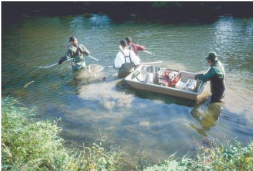
Organochlorine pesticides (many of which are now banned) are persistent in the environment. Trace amounts are present in streambed sediment and fish. Fish are collected for study by a team of biologists using equipment like this barge-mounted electroshocker. (Photograph by Steven F. Siwec, U.S. Geological Survey.)
