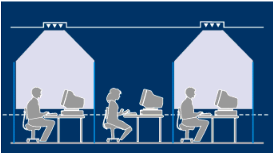
After adding partitions to the room, the spacing between fixtures becomes too wide.
