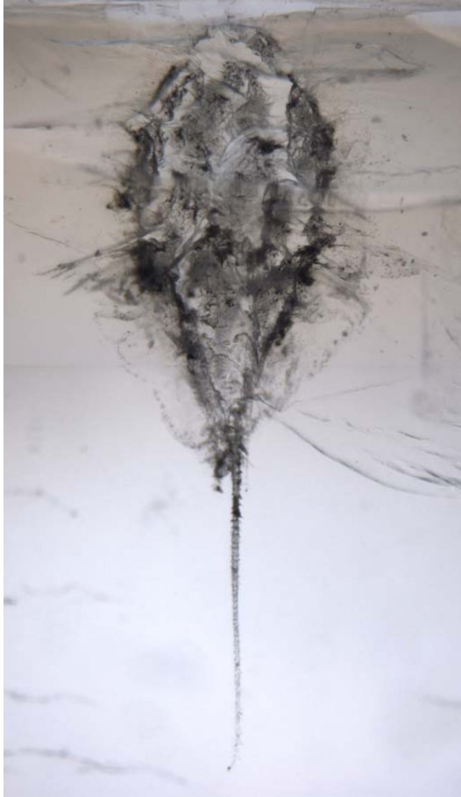
Figure 1. A bulbous track (C2054,0,35) in aerogel from the Stardust samples. The particle entered the aerogel at the top, shed part of its mass through interaction and deceleration in the aerogel, and the larger intact grains traveled the furthest, with solid mineral grains typical at the terminus of the track. The total track length here is ~11 mm.
