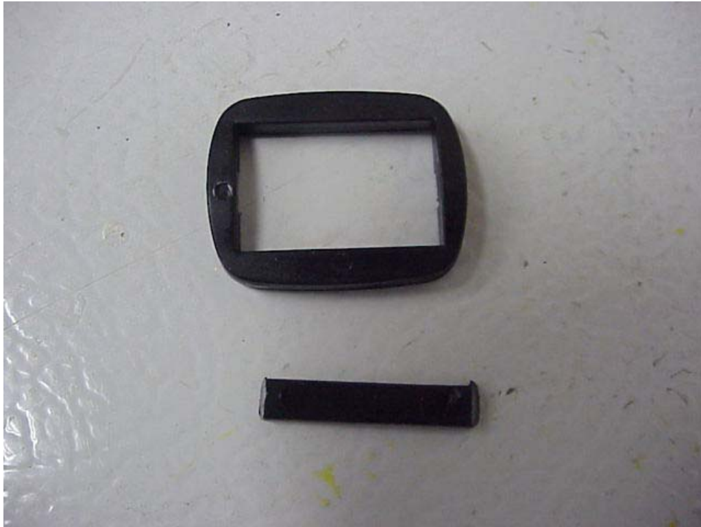
Helmet Photograph 9. Broken Retention System Component Kerr, H205 BLK, M
