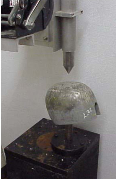
SwRI Helmet Test Equipment Photo 4. Penetration Resistance Tester Configured for Crown Locations
