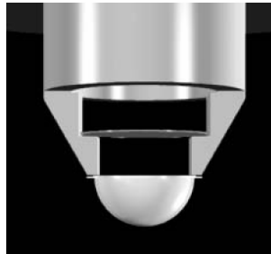
FIGURE 2. Open target mount with hemispherical capsule on 30- \mu\text{m} -thick gold disc.
