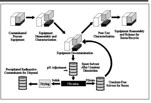
► Cleaning of surface contamination on process equipment to a level allowing for reuse of the process equipment components or materials
