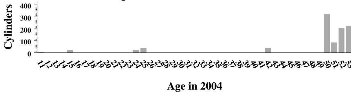
Figure 31. Minimum thicknesses (top) and age distribution (below) for ETTP/PGDP/PORTS thick top cylinders.
