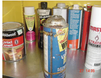
Top Left—Don't store chemicals near food or eating supplies Top Right—Improper labeling Lower Left—Rusted can may become a danger due to leaking Lower right—Nothing. Chemicals correctly separated in bins.
