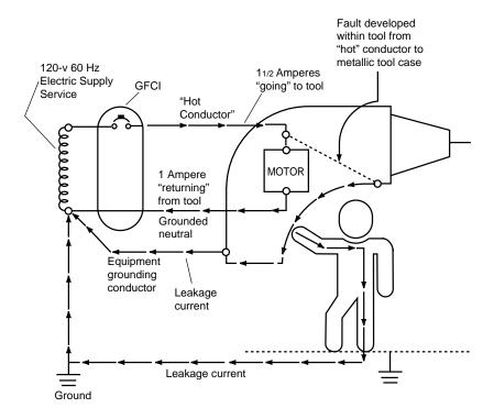
GFCI monitors the difference in current flowing into the "hot" and out to the grounded neutral conductors. The difference (½ ampere in this case) will flow back through any available path, such as the equipment grounding conductor, and through a person holding the tool, if the person is in contact with a grounded object.
