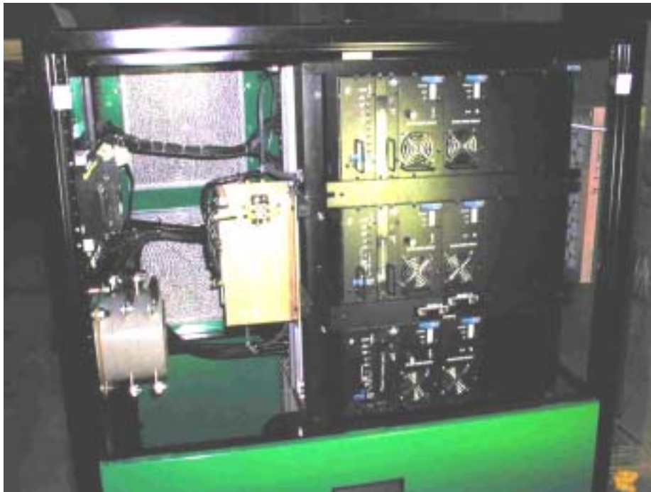
Figure 2-6. Right side of the electronics cabinet (Shows the power electronics, boost converters, and inverters)
