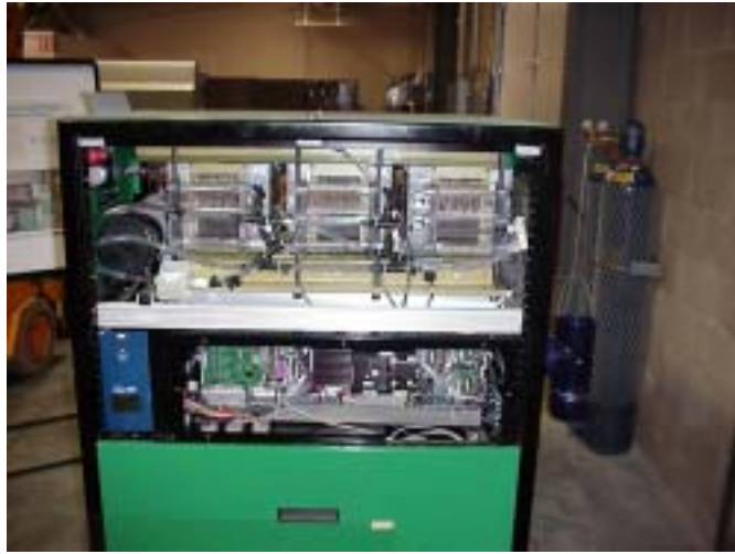
Figure 2-3. Right view of the fuel cell cabinet and hydrogen tanks (The top section contains the three stacks and associated tubing for hydrogen and water; the middle section contains control circuitry)
