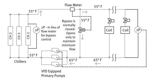
Figure 3 Primary Only Chilled Water Pumping Schematic
