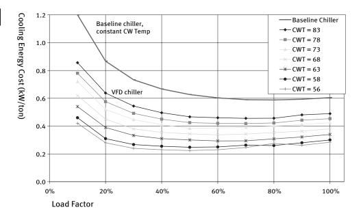
Design Cooling Water System to Operate near Design Chilled Water delta T at Part-load
