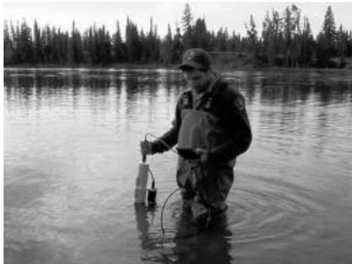
NPS Aquatic Ecologist Jeff Arnold lowers a monitoring probe into the Yellowstone River as part of the long-term water quality monitoring program, August 2002.
