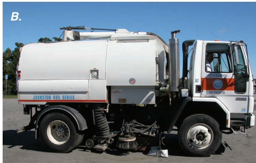
Figure 4. A, Pelican Series P mechanical sweeper and B, Johnston 605 Series vacuum sweeper, used in the evaluation of sweeper efficiencies.
