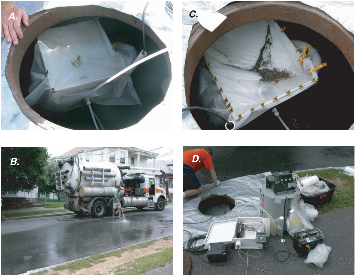
Figure 3. A, Street-dirt collection device installed in the Query Street catch basin; B, Query Street washing with the Vector machine; C, collection of wash water with entrained street dirt as part of the street-dirt accumulation experiments; and D, equipment used to measure discharge and sample wash water, New Bedford, Massachusetts.
