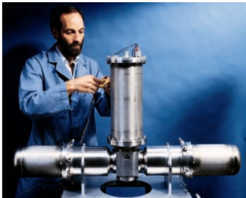
Stirling Technology Company engineer readies the cryocooler. NASA requirements called for low-temperature equipment to run sensors to achieve refrigeration levels for a space-rated freezer.
