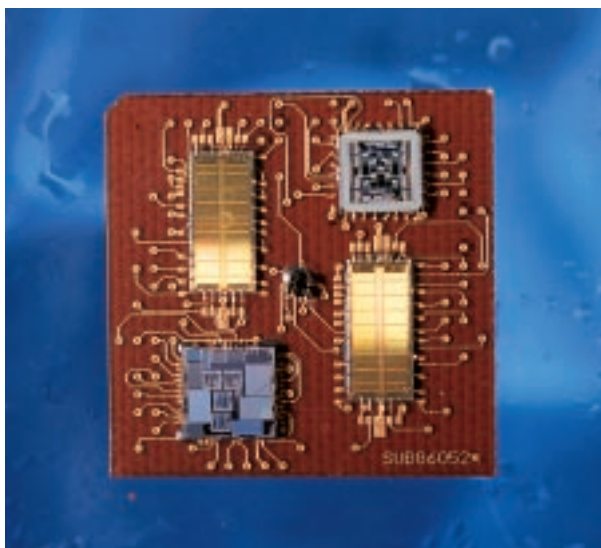
High-value electronic circuitry can be overcoated with an inorganic moisture barrier. Shown is a circuit board, replete with an alert chip (center) that signals if moisture has penetrated the circuit surface.
