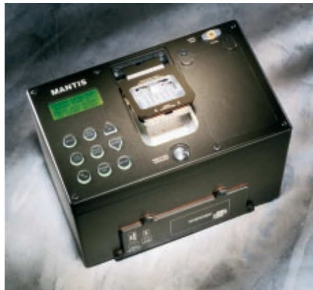
NASA-supported research helped in the creation of micromachined pumps. This appliance is integral to a number of Research International products, like this highly-sensitive portable unit that detects toxins, explosives, and chemical contaminants.
