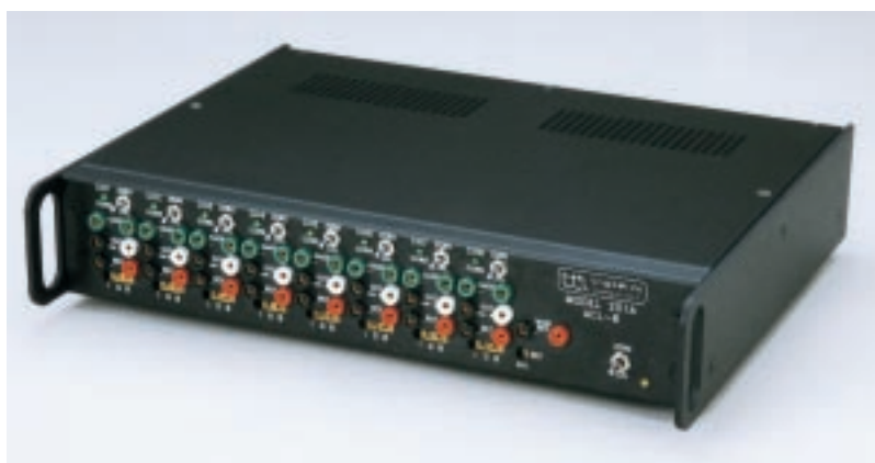
Trig-Tek measurement device incorporates the NASA-invented Anderson loop electrical circuit. This measuring circuit is far more accurate than commonly used test procedures.
