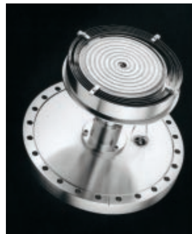
Substrate heating unit is made of inconel. High temperatures reached by the heater are key to depositing superconducting thin films.
