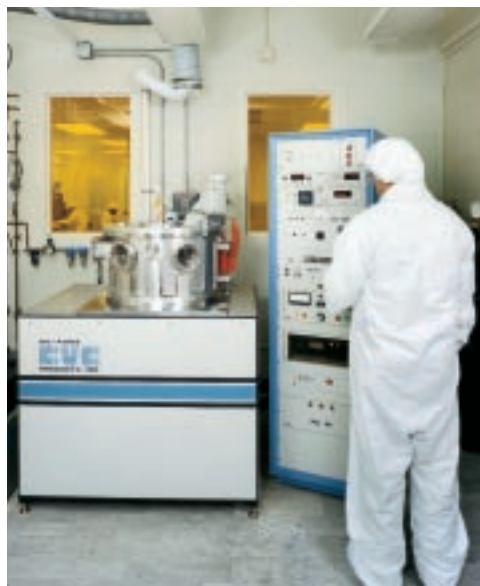
Specialist prepares CVC's system for depositing superconducting thin films.
