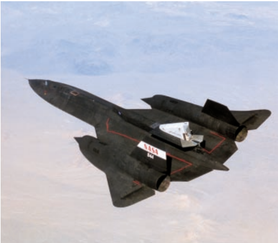
Dryden is flight testing the Linear Aerospike SR-71 Experiment (LASRE), which is designed to gather data on the aerospike's exhaust plume as it travels through the transonic region of flight (just below to just above Mach 1).
