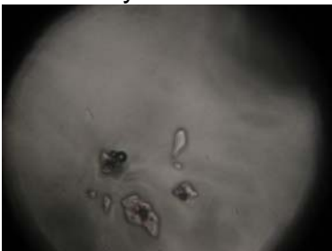
Figure 17. Low Flux E-glass showing clusters of unmelted batch silica grains (cristobalite)
