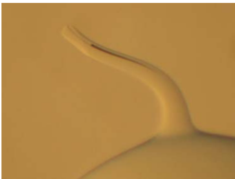
Figures 8a & 8b. Dark Lines In Fiber Tips Are Hollow Filaments (seeds/bubbles) That Likely Caused The Fiber to Break Out
