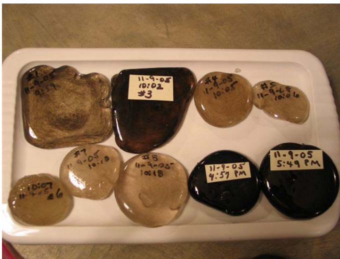
Figure 20. Suite of Low DK Glass patties produced during the plasma melting trial
