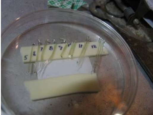
Fig. 5 Glass Beads with Defects Collected During Fiberizing Trials
