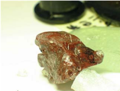
Figure 15. AR Glass showing oxidized molybdenum from startup glass
