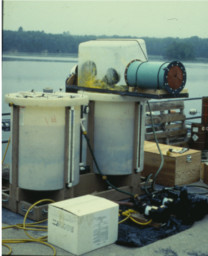
Figure 6-2. Bayluscide® 70% Wettable Powder mixing and application apparatus. The powder is mixed with fresh river water to form a slurry to facilitate application of the formulation to the river. Note the apparatus is self-contained to minimize applicator exposure to the lampricide formulation.
