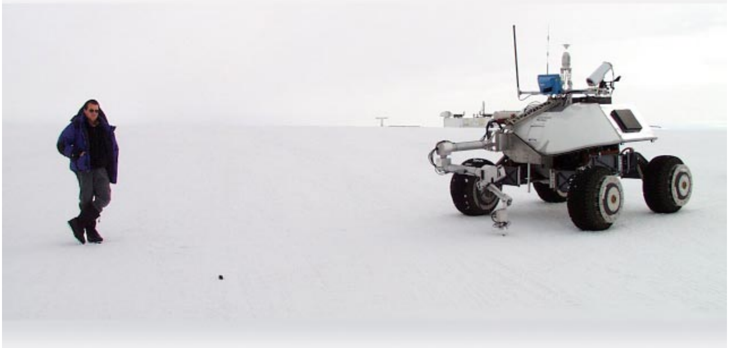
Ben Shamah, a Carnegie-Mellon research engineer, monitors Nomad on a trial run near Williams Field. The robotic meteorite hunter contains all the technology needed to locate and analyze potential space rocks. Photo by Josh Landis.
