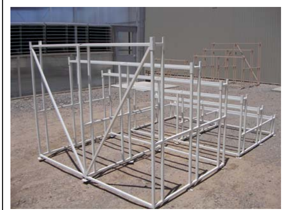
Figure 2. A welded steel frame made of 1" square tubing for bioreactor support.
