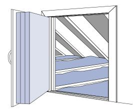
Add R-value to a knee-wall door by adhering rigid insulation boards (sandwiched together with construction adhesive and screws) to the back of the door. Pay special attention to the clearance between the insulation and the door frame and air sealing details.
