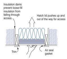
To create the hatch, the installer should cut a plywood piece or save the ceiling drywall piece that is cut out for the hole. To ensure a tight fit, securely fasten the trim around the hole to the ceiling and make sure that it is flat and level. An uneven base can cause air leakage. Weatherstripping can be installed either on the hatch itself or on the inside of the trim or base where the hatch rests. Adding a latch bolt will help ensure a tighter seal.
