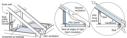
The attic knee wall is often underinsulated and leaky. Install adequate insulation and air seal around the living space for continuity in the building envelope when addressing the knee-wall door.
