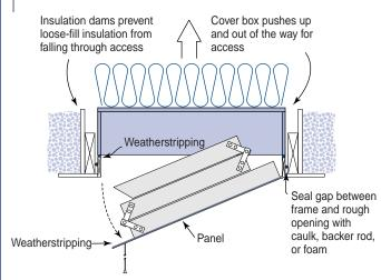
An attic stair cover box is made from rigid insulation. It drops down from the attic side to seal and insulate the pull-down stairs.
