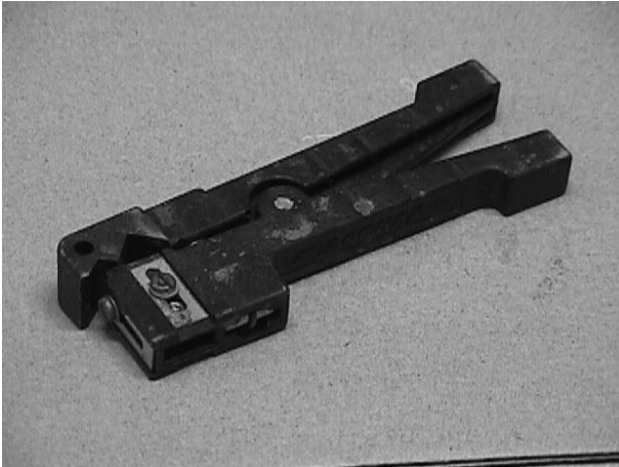
Fig. 3-3. A coaxial cable stripper sold by Radio Shack. The blade on the left side (visible on top of stripper in this view) is set to cut through only the outer cable insulation. The blade on the right side (not visible here) is set to cut through the outer insulation, cable braid, and inner insulation, but not through the center wire of the cable.
