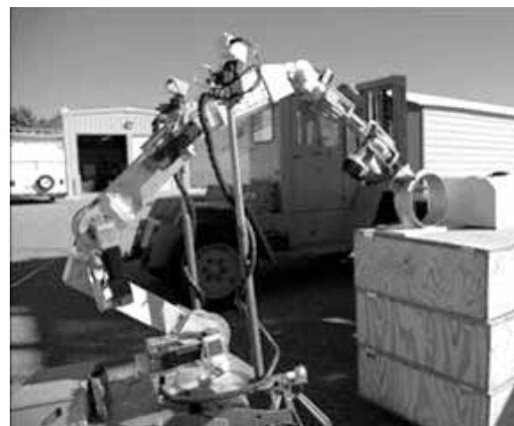
HOW DO YOU GET to Carnegie Hall? Practice, man, practice. Here, M2 (Mighty Mouse) practices the complex drilling routine it will follow to free up the stuck radiation source at White Sands.
