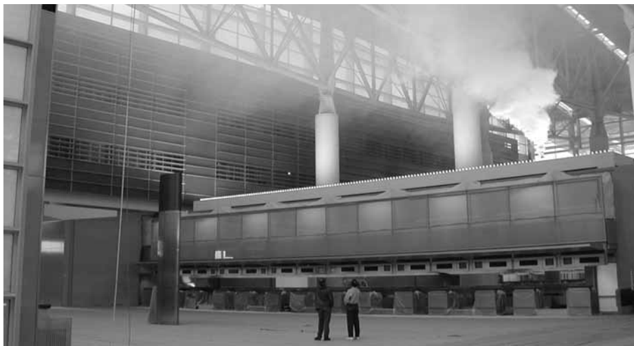
THE SECURITY GUIDELINES developed by Sandia and LBNL were based on many data sets, including information gained from tests at San Francisco International Airport. The smoke dispersal test shown above was conducted several years ago in a new, unoccupied wing of the airport.
