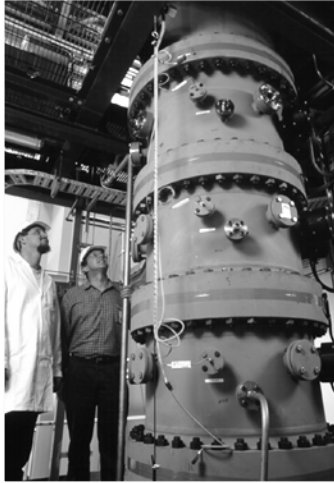
Daniel Henderson and David Harris with coal-gasification reactor. Courtesy: CSIRO Energy Technology
