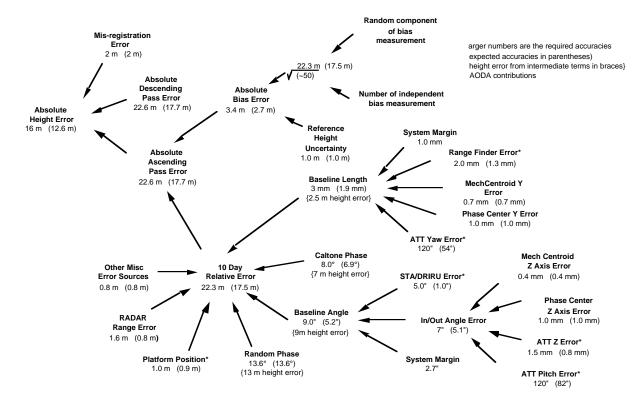
Figure 4 - SRTM Height Error Budget
