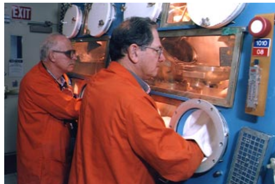
Figure 2. To be suitable for most disposition methods, the excess weapons plutonium must first be converted into plutonium oxide by various hydride/oxidation (HYDOX) methods. The prototype HYDOX furnace design originated at Livermore and has been used to test various HYDOX process options. Livermore technicians William Kuhl (left) and Terry Ludlow assemble a HYDOX furnace in a glovebox. The unit will be used for further testing at Los Alamos National Laboratory.
