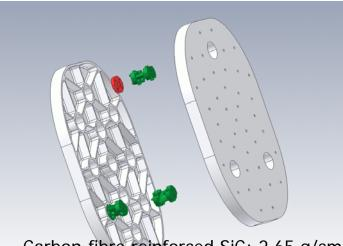
Carbon-fibre reinforced SiC; 2.65 g/cm<sup>3</sup> E-Modul: 111 GPa; expansion coeff: 2E-06 / K
