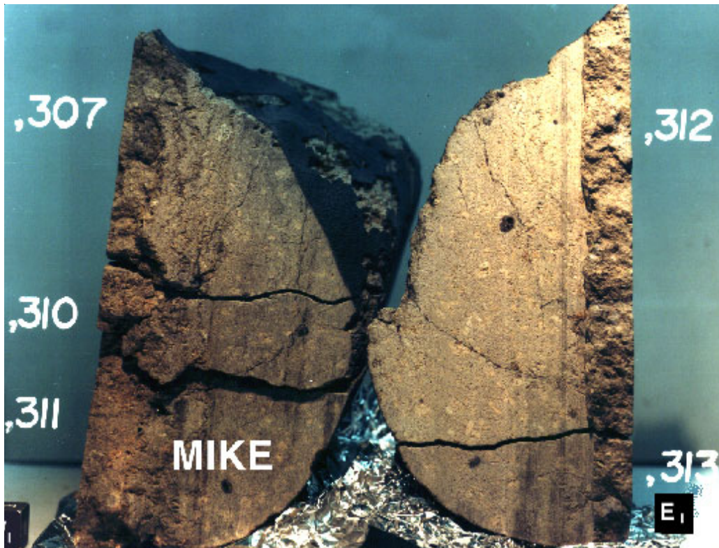
Figure IX-30. Sawn face of EETA79001 showing opposing pieces. Note the thin glass veins and small glass pods. NASA photo # S90-34042.
