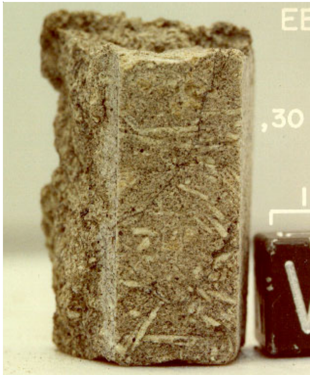
Figure IX-7. Close-up photo of sawn surface of EETA79001,30 illustrating the basaltic texture of lithology B. Cube is 1 cm. (NASA # S81-25238)
