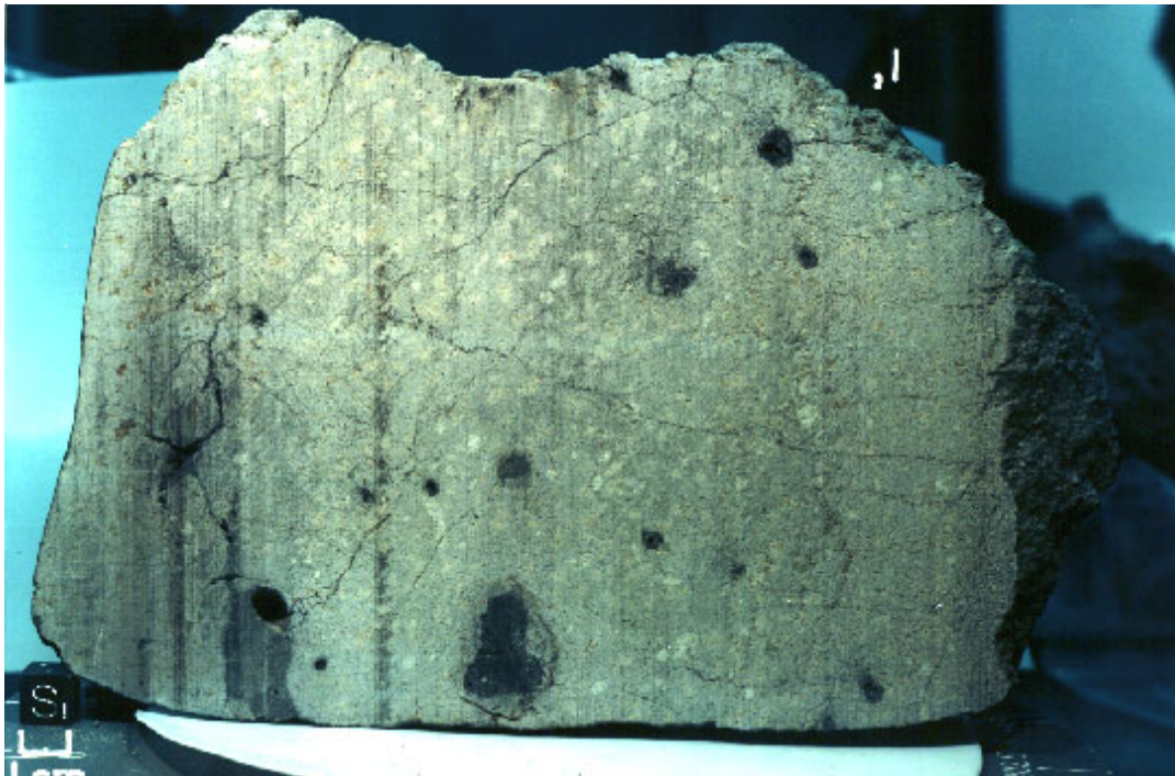
Figure IX-26. Sawn face of EETA79001,1 after first saw cut (NASA # S80-37631). See figures IX-21 and IX-23. Sawing was done dry, with a steel band saw.
